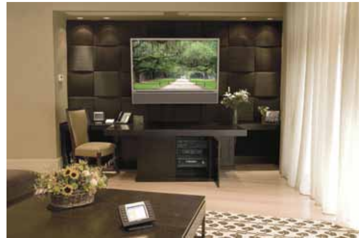
A rack that used to contain large audio and video matrix switches, a total home control central processor, banks of TV set-top boxes, and CD and DVD players now has shrunk to a small fraction of its original size because entertainment content can now be streamed over the home network from local hard drive sources or the internet cloud. Pictured is a Middle Atlantic SRSR Series sliding rotating rack in an install performed by Intra Home Systems.
